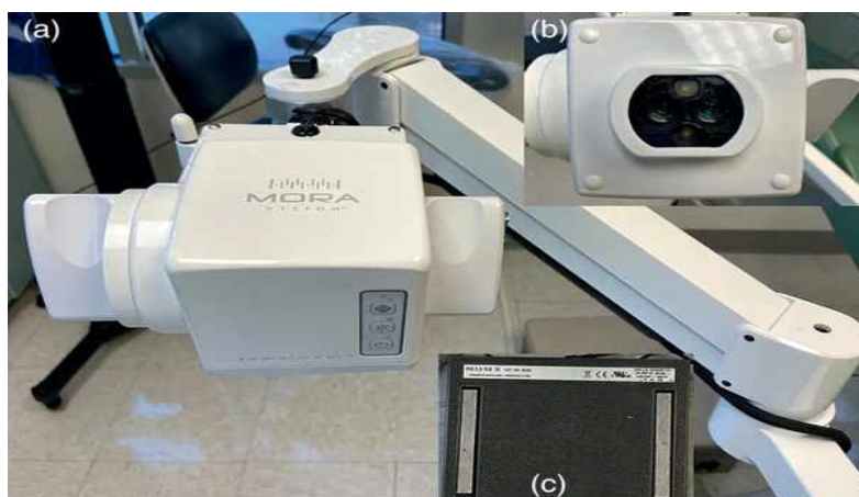
Figure 3 : The Mora Vision video imaging system is an example of digital illumination, magnification, and recording during dental (including endodontic) procedures: (a) the main mount and arm system of the camera; (b) the lenses and illumination interface of the multi-lens video camera system; (c) the foot pedal.
